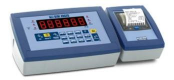
Digital weight indicator for weighbridge management. Extremely simple and intuitive, easing the user with the weighing operations. Fitted with database of 99 open input weighs and database of 30 quickly recallable tares. Fitted with attached thermal printer. CE-M approvable (OIML R-76 / EN 45501).
