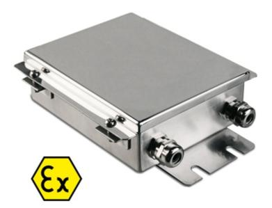
Stainless steel junction box with IP66 protection from water and dust, and fitted with an intrinsically safe electronic board for junction and equalisation of load cells. Terminal boards with screws for easing th connection of the load cells and signal adjustment trimmer, for an accurate and reliable equalisation. Marking: ATEX II 2G Ex ib IIC T6 Gb for gases. ATEX II 2D Ex tb IIIC T115°C Db IP65 for dust.
