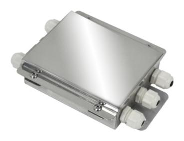
Stainless steel junction box with IP65 protection from water and dust, and fitted with electronic board for junction and equalisation of 4 or 6 load cells. Terminal board with screw for easing the connection of the load cells and the signal adjustment trimmer, for an accurate and reliable equalisation.
